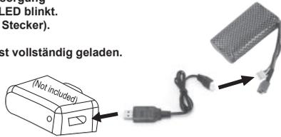
**ALWAYS charge the battery outside the model, to avoid overheating during charging, always use a fireproof base!**
